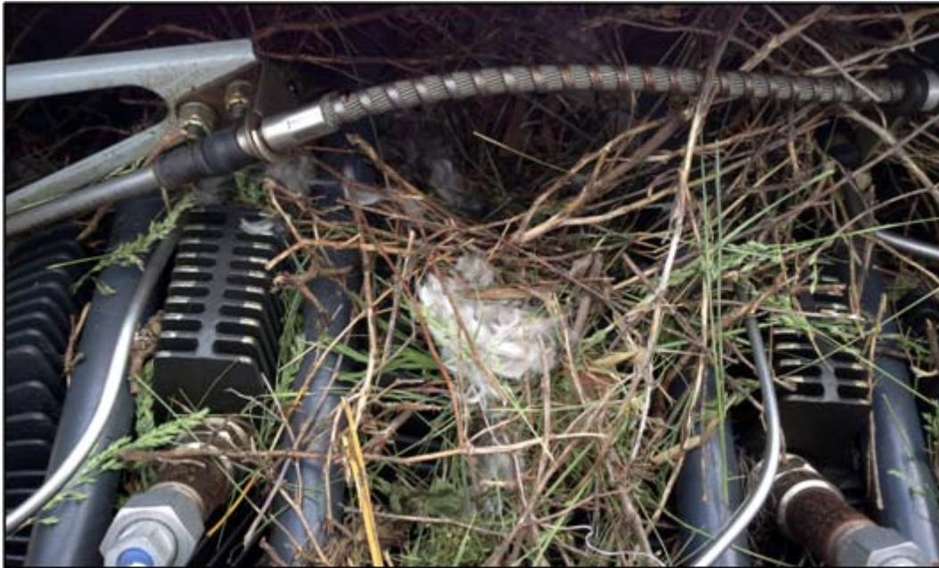
Cooling airflow blocked by the nesting materials can cause critical aircraft systems to overheat, and can be a flight safety concern too. A nest left in close proximity to the engine exhaust system can catch fire, or could interfere with flight control movements.
